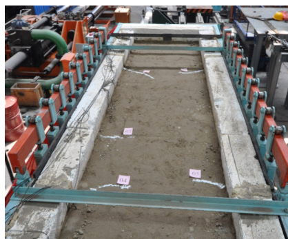
图 7 一致激励下自由场土体的破坏 Fig.7 Damage of the soil under the uniform excitation
